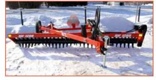
The Rite Way 1200HD rock windrower delivers rocks to the windrow more efficiently with its three-row spiral design. It features hard surface replaceable teeth.
