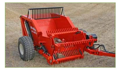
The RR900ST has a three-bat shock protected reel system and can remove rocks from 2" to 28" in diameter and up to 55" in length. Its ample, 60" picking width removes more rocks in fewer passes and its 3.2 cu yd capacity bucket lets you pick more rocks before dumping.
