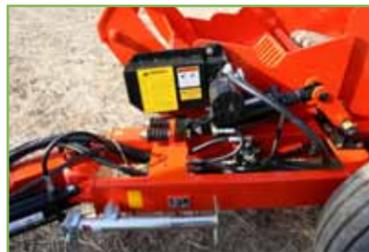
The RR250ST has a two-bat shock protected reel system and can remove rocks from 2" to 24" in diameter and up to 45" in length.
