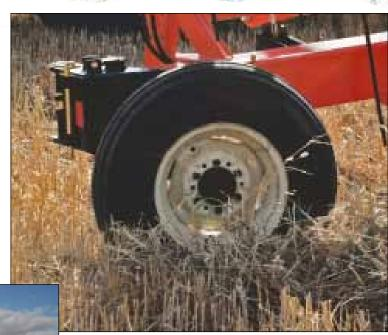
At the touch of the hydraulic lever, the Field Transport Pivot Wheel System eases the harrow bar in or out of the transport postion
